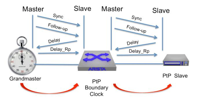
As an example, if a master clock is capable of supporting 100 devices, and each boundary clock can support an additional 100 devices, the PTP implementation can scale by 100X by implementing a single tier of boundary clocks in the network, achieving a much larger network than with the grand master clock alone. This also prevents having to provision numerous grand masters at different points in the network. As the boundary clock becomes the authoritative
