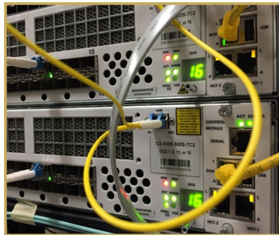
Front of units under test: Cloud Xpress CX-100E (bottom) and Arista 7280SE-68 (top)
