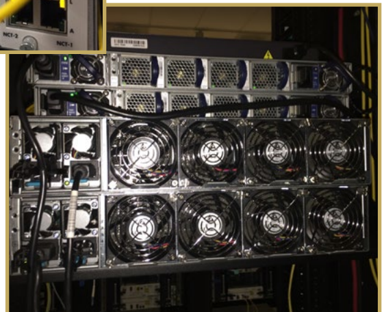
Rear of units under test: Cloud Xpress CX-100E (bottom) and Arista 7280SE-68 (top)
